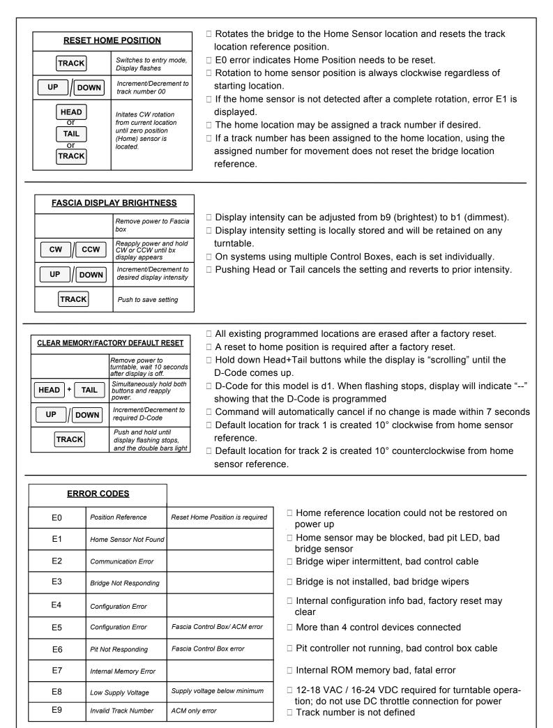
E0 Position Error can be cleared by pushing any key. Service track locations will not be correct until a reset of the home position is done. Other errors will clear automatically when the cause is corrected.
