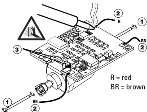
Loosen the motor from the circuit board.
