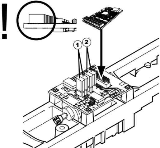
① Jumper enables you to reverse the direction. This is necessary if the headlights go on in one direction and the locomotive runs in the other direction.
