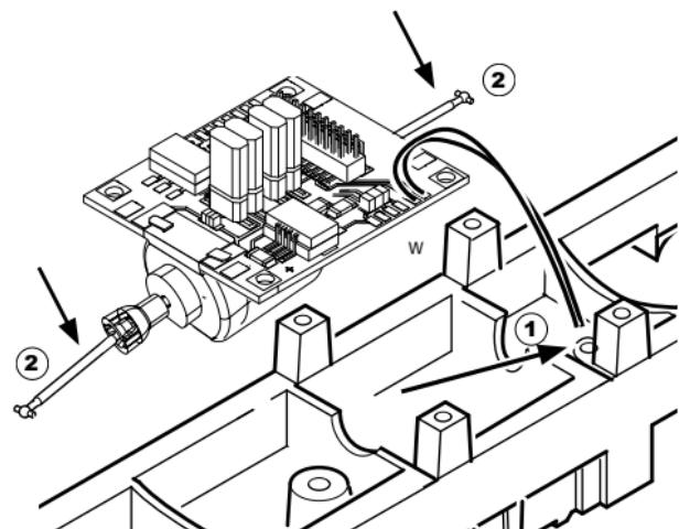
Screw the circuit board in place, solder the wires in place and plug the ribbon cable back in,
