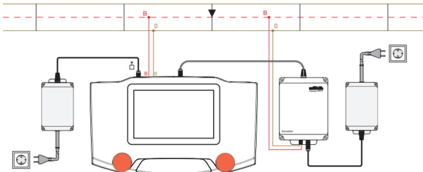
If you want to operate additional 60175 Boosters with the Central Station, then you can connect the 60125 Terminal to the Central Station and connect up to four Boosters to each Terminal.
