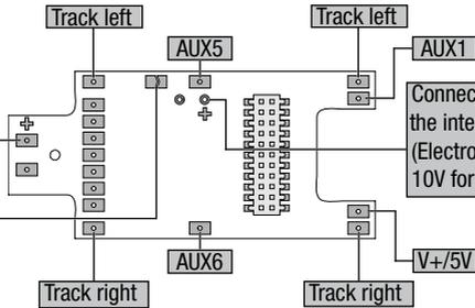
Connection of a buffer capacitor for the interior lighting (Electrolytic capacitor 220µF; 10V for DC and AC)
